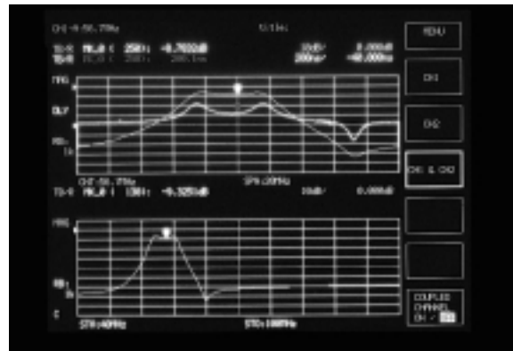
Spurious measurement using alternate sweeping
