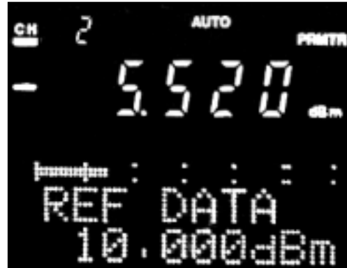
Reference data input (MT9810A display)
