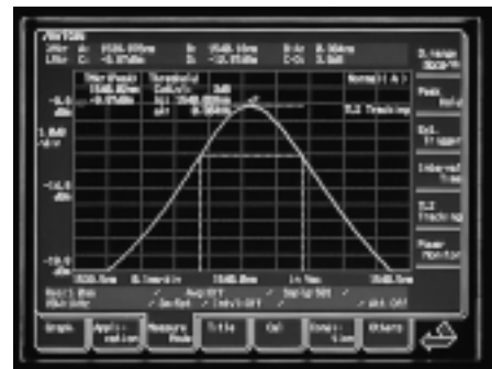
Screen A: FWHM measurement example
