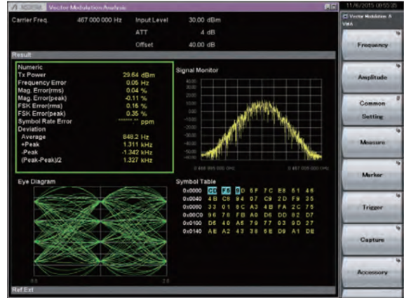
4FSK Modulation Analysis Measurement Example
