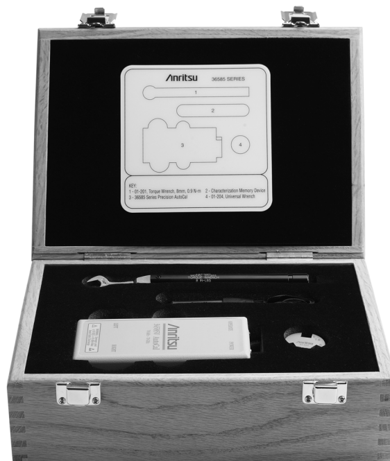
36585 Series Precision AutoCal Calibration Kit
