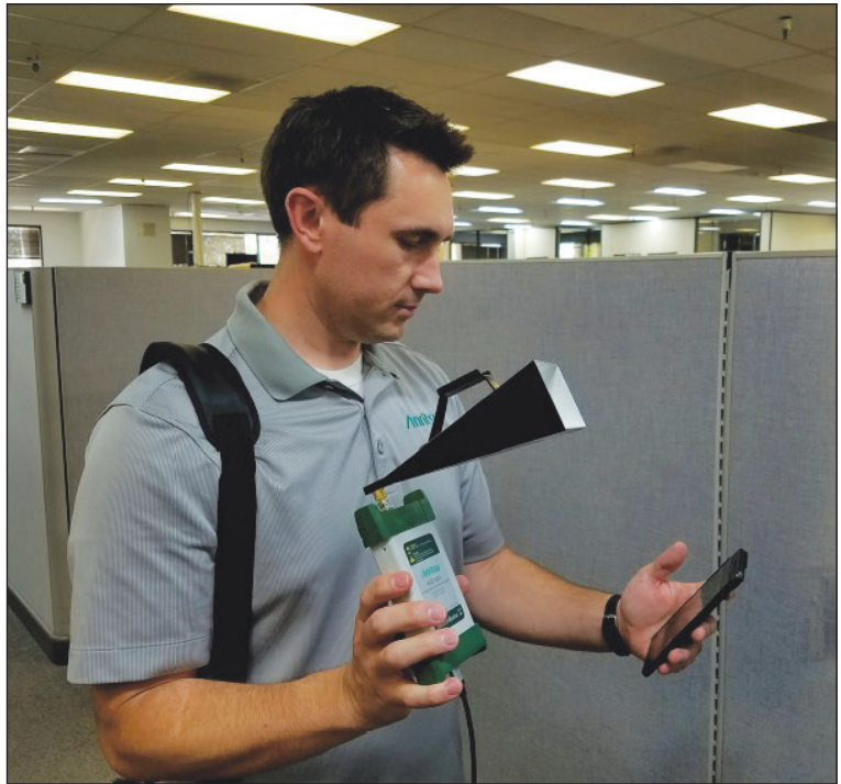
Figure 4. Millimeter-wave indoor coverage mapping solution.
